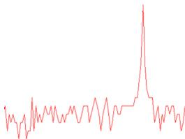
This feature is used to inhibit high amplitude electrical noise from outside the vibration monitoring system from impacting the performance of the vibration transmitter system. It temporarily suppresses high amplitude, short duration, typically less than 50 millisecond vibration spikes - like those induced possibly by a portable radio when keying the RF device.
