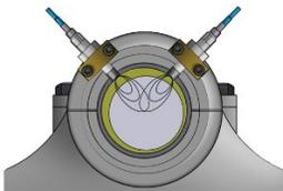
Cross Talk Elimination is used when proximity probes are close together, typically less than 25mm. This feature is used on one of the probes that could interfere electrically with another probe close by. One can shift the transmitter oscillation frequency making it different from the adjacent probe, thereby, preventing Cross Talk interference.
