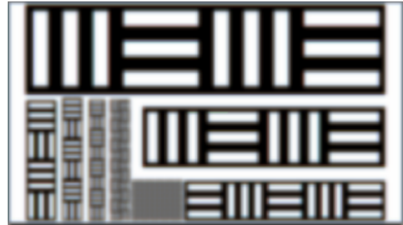
Resolv4K Zoom @ 4.5X High Mag 8.9MP Sensor – 0.76\mu\text{m} / pixel 3.56mm FOV – 5.20\text{mm}^2 Area (3.25X more)
