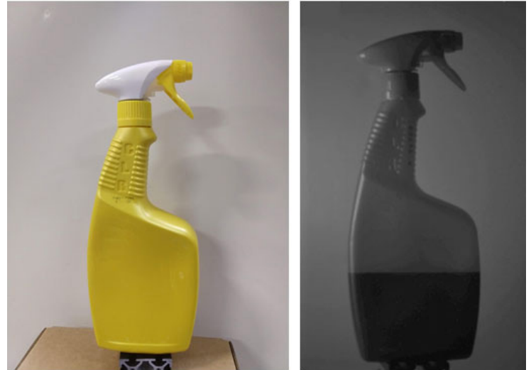
Figure 3 - A 1550 nm SWIR light can enable a SWIR camera to see through a plastic container and show the fluid level.
