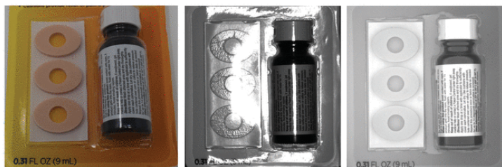
Figure 8: Examples of imaging through clear plastic package (left), using diffuse ring light (center) and flat dome light (right) are pictured here.
