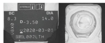
Figure 12: Examples of imaging wrinkled foil contact lens package (left), using diffuse ring light (center) and flat dome light (right) are shown here.
